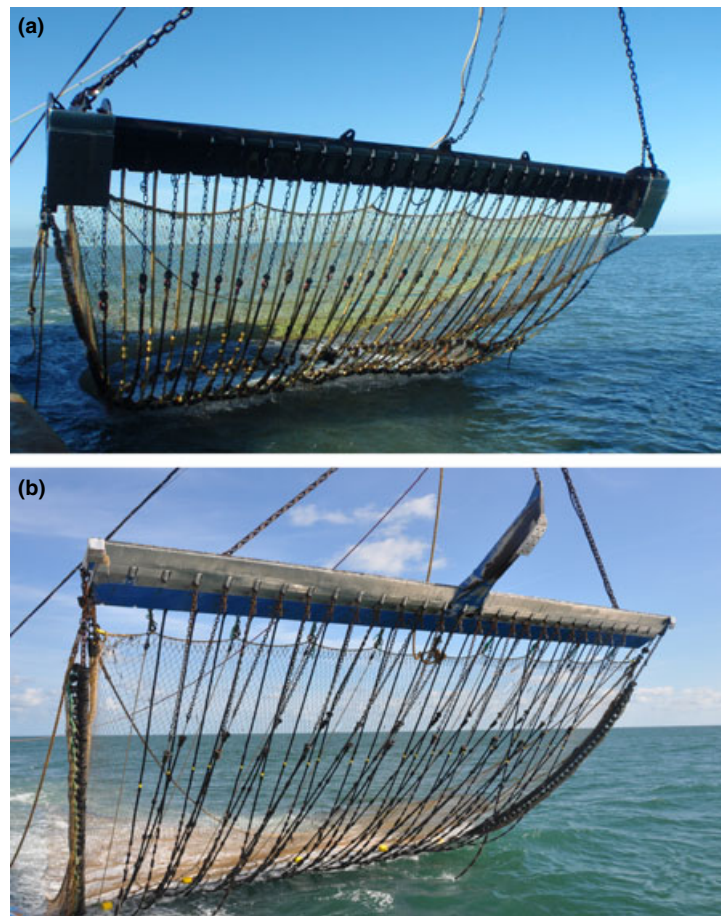
Figure 2 The Delmeco pulse beam with beam and trawl shoes (a) and the HFK PulseWing with the wing and the runner in the centre (b).
