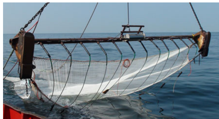
Figure 4 The Hovercran with 9-m beam and trawl shoes. The cylinder fixed on the middle of the beam is the pulse generator.
