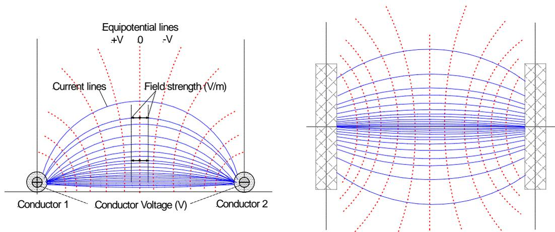
**FIGURE 4.2. CURRENT FLUX LINES BETWEEN A PAIR OF CYLINDRICAL CONDUCTORS IN THE VERTICAL AND HORIZONTAL PLANE. CURRENT LINES ARE DENSELY PACKED AT THE CENTRE AXIS PERPENDICULAR TO THE CONDUCTORS. NOTE THAT AREAS OF MINOR FIELD STRENGTH OCCUR BELOW AND ABOVE THE CONDUCTORS.**
