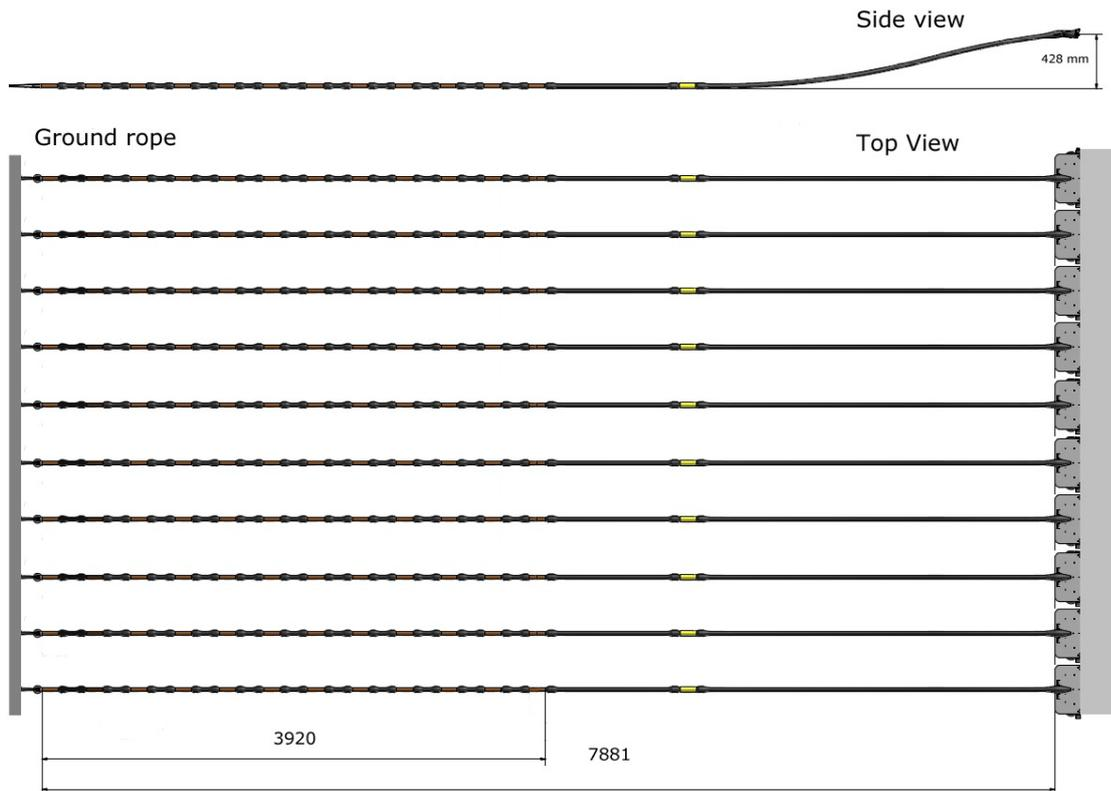
**FIGURE 4.1. RIGGING OF HFK ELECTRODES OF A 4 M BEAM TRAWL. THE TOP PANEL SHOWS THE SIDE-VIEW WITH A VERTICAL TRAWL OPENING OF 0.43 M. THE BOTTOM PANEL SHOWS THE TOP-VIEW OF THE 10 ELECTRODES RIGGED BETWEEN THE WING AND THE GROUND ROPE. EACH ELECTRODE CONSISTS OF A MAXIMUM OF 12 CONDUCTOR ELEMENTS, EVENLY PLACED OVER A LENGTH OF 3.92 M, THAT ARE IN CONTACT WITH THE SEA BED. AN ISOLATED JOINT (MARKED YELLOW) IS USED TO EXCHANGE ELECTRODES.**
